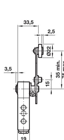
Mechanism may be operated either side of centre line.
