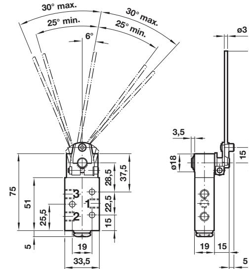
Mechanism may be operated either side of centre line.
